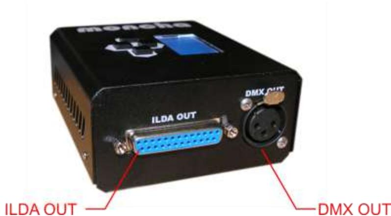
There is ILDA output for laser and DMX output on the rear side of the Moncha.NET device.
