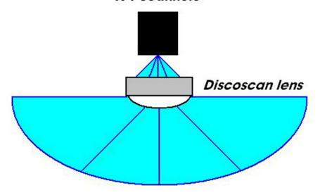
180 by 360 scan field (projecting downward from the horizon)
