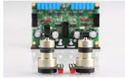
ScannerMax 506 for precise and reliable 40kpps scanning. 90kpps scanning is optional.
